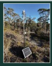
By integrating a LoRa gateway, this advanced monitoring system extends its communication capabilities, enabling seamless connectivity with deployed field sensors across vast distances. With a range exceeding 40 km, the network ensures wide-area coverage, making it highly effective for monitoring planned burns and maintaining control over large, remote areas.
